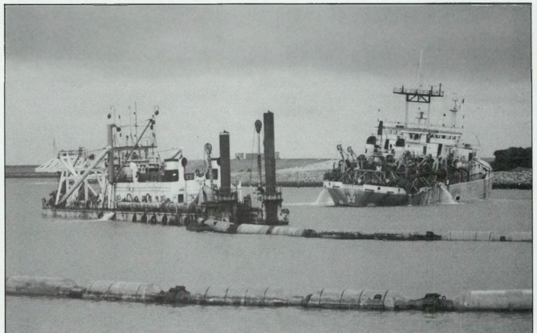
Jan de Nul's trailer-suction hopper dredger "Sanderus" dumping sand for re-dredging and pumping to the western breakwater area by the cutter dredger "Ortelius".
