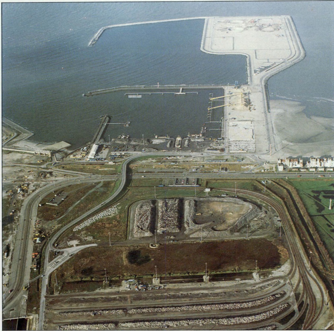
Picture showing the east stock area with its graded piles of stone, the work harbour for use by the various contractors, and the start of the work on the L.N.G. terminal area.
