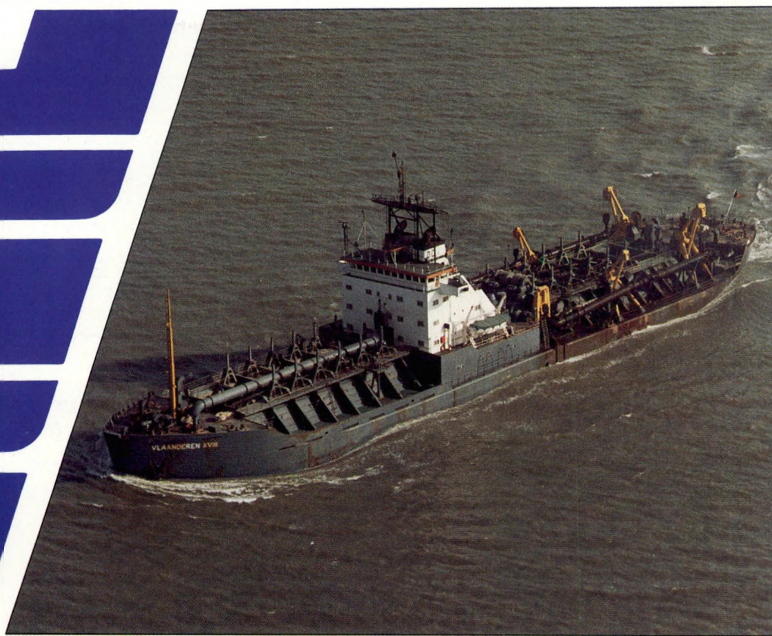
Largest Trailing Hopper Suction Dredger in the world, Vlaanderen XVIII, dredging the entrance channels at Zeebrugge – Belgium.
