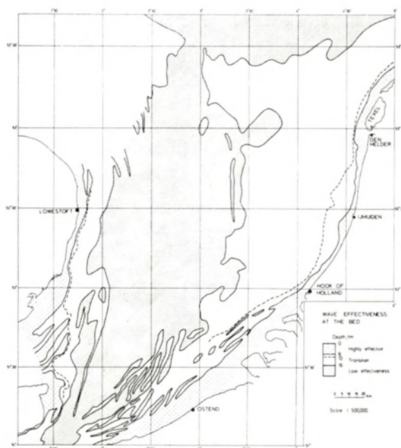
Fig 86. Theoretical wave effectiveness at the bed from calculations based on the data of DRAPER (1967) by McCave (1971).
