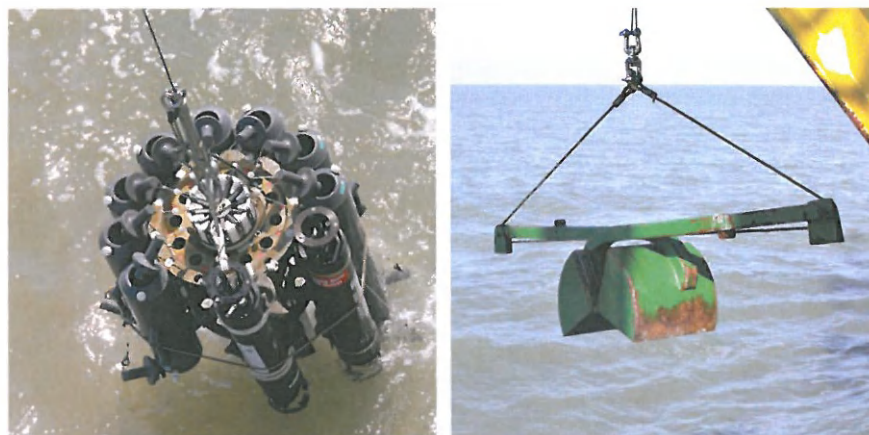
Figure 1.2: Niskin bottles mounted on a carousel for water sampling (left) and a Van Veen-grab used for sediment sampling (right).
