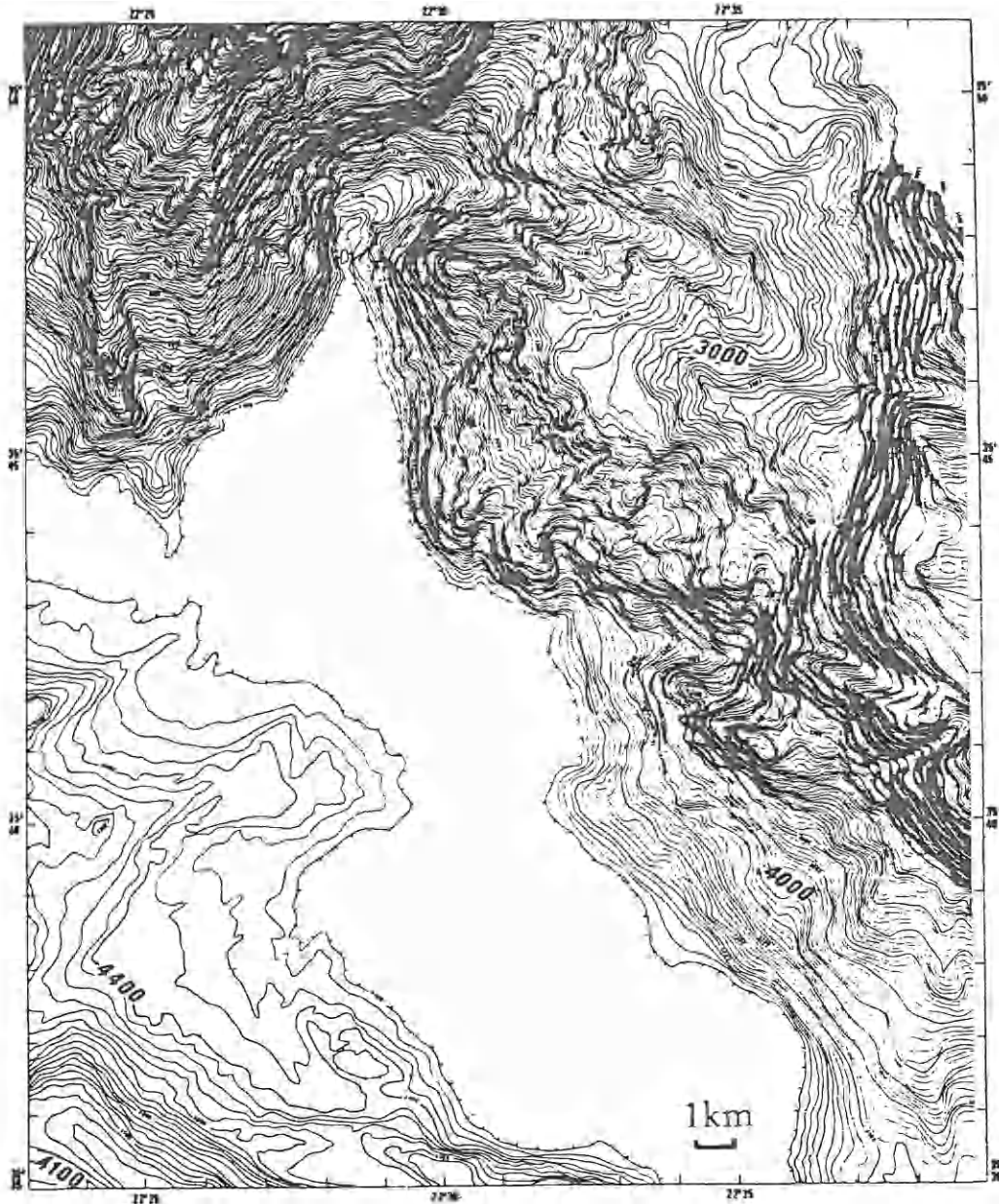
Fig. 1.4. South Matapan Trench, deepest Mediterranean seafloor, mapped with a multichannel (Sea-Beam) system (after Huchon et al., 1982; kindly provided by X. Le Pichon, Paris). Contour interval 20 m (corrected). Example of an abyssal plain on a segment of the Hellenic Trench, southwest of the Peloponnesus, at the contact between the Aegean land-mass and Mediterranean Ridge. The flat bottom is
