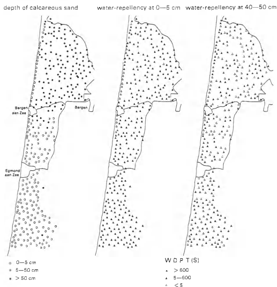
Fig. 10: Depth of calcareous sand and degree of water repellency at 0–5 cm depth and at 40–50 cm depth in dune sands north and south of Bergen. (DEKKER & JUNGRIUS, 1990)
