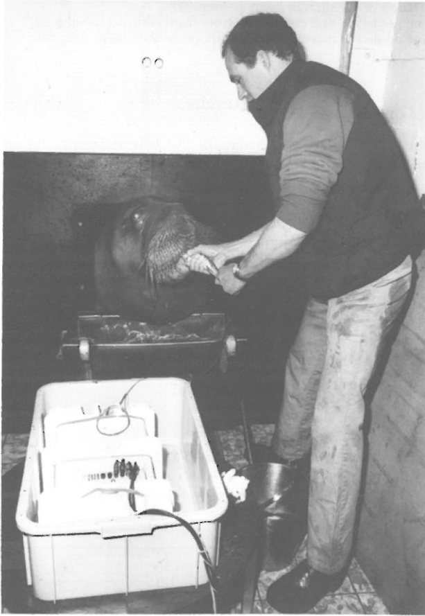
Fig. 1. The walrus sucking a fish containing the pressure transducer. The hole in the door is 50 × 50 cm (Photo: HENK MERJENBURGH)
