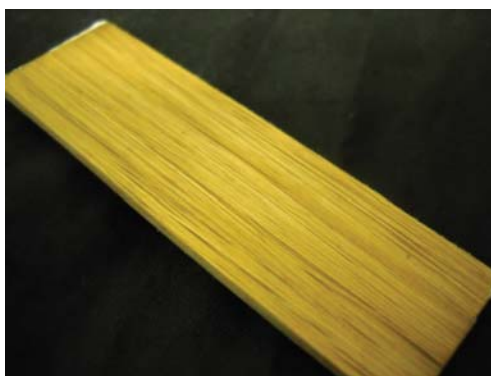
Figure 1: Unidirectional bamboo fibre composite with thermoplastic matrix.
