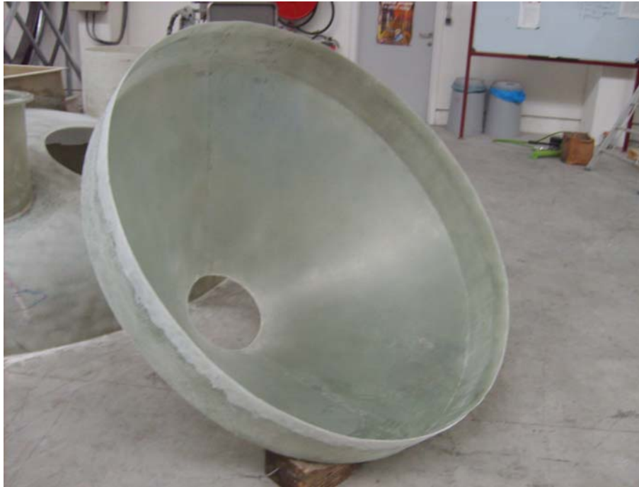
Figure 8-33 One of the four spray up cones.
