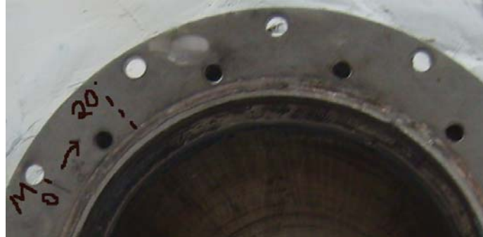
Figure 8-46 Marked meridians on flange.
