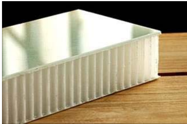
Figure 4-14 Sandwich structure with a honeycomb core.
