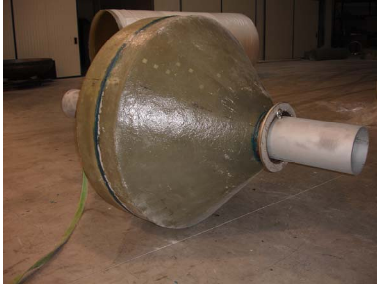
Figure 8-36 Assembly of two cones, one inner tube and the steel tube.
