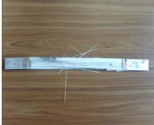
Figure 4-19 Test sample tensile 0 degrees after fracture.
