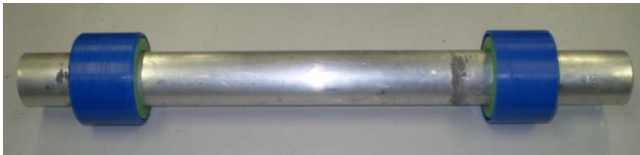
Figure 7-40 Aluminium tube with polyethylene and polypropylene parts.
