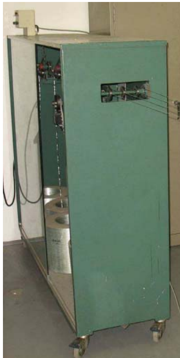
Figure 6-3 Closet with bobbin holders and pre-tension mechanism.
