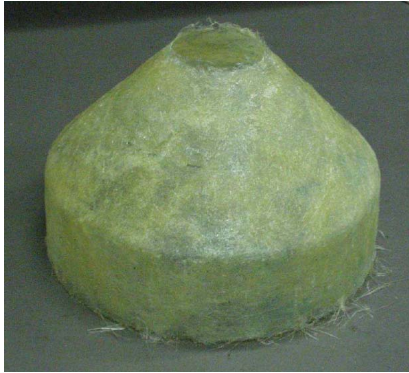
Figure 6-26 One of the two cones made with chopped fibres and resin [3].
