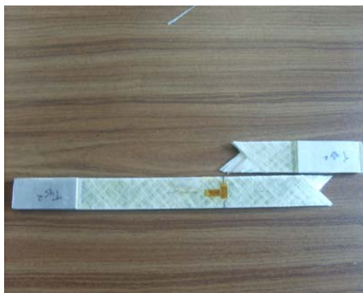
Figure 4-21 Test sample tensile 45 degrees after fracture.
