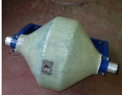
Figure 7-41 Laboratory scale point absorber with connection for the ladder [2, 15, 16].
