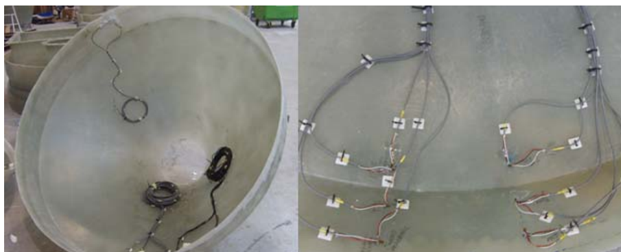
Figure 8-43 Pictures of the mounted inner strain gauges.
