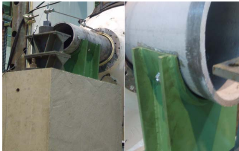
Figure 8-26 Rectangular concrete block and small support (green).
