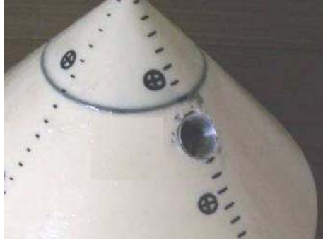
Figure 7-9 Position of the pressure sensor.
