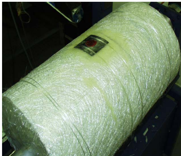
Figure 7-28 PU cylinder with chopped fibre layer and curved plate for the pressure sensor [2, 15, 16].
