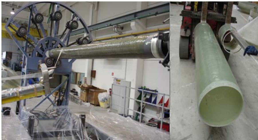
Figure 8-35 Production of composite tube (left) and finalised tube (right).
