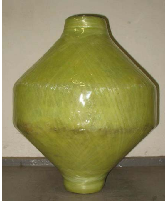
Figure 6-32 Result of the first produced laboratory point absorber on the filament winding machine[3].
