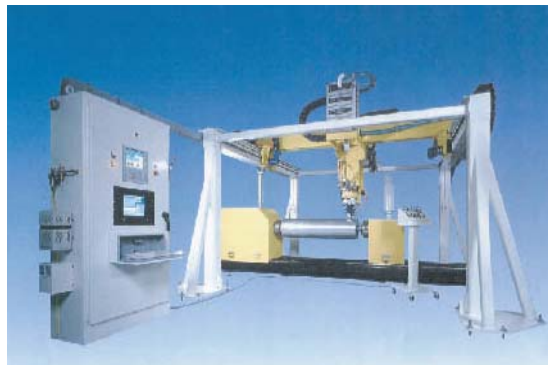
Figure 4-2 Example of a 6-axes winding machine [4].
