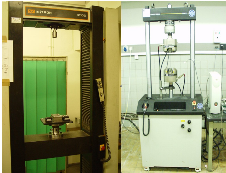
Figure 4-17 Mechanical instron (left) and the hydraulic instron (right) in the lab of Ghent University.
