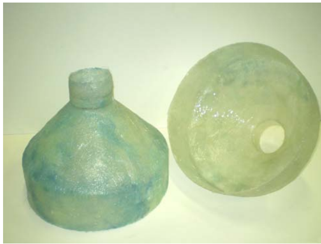
Figure 7-39 Two cones made with chopped fibres.
