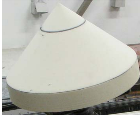
Figure 7-5 Produced cone in polyurethane (PU).
