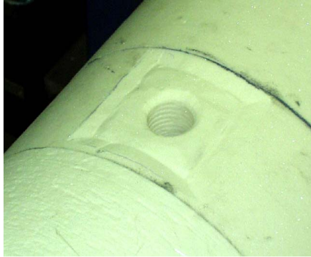
Figure 7-27 PU cylinder: preparation of the location for the pressure sensor [2, 15, 16].
