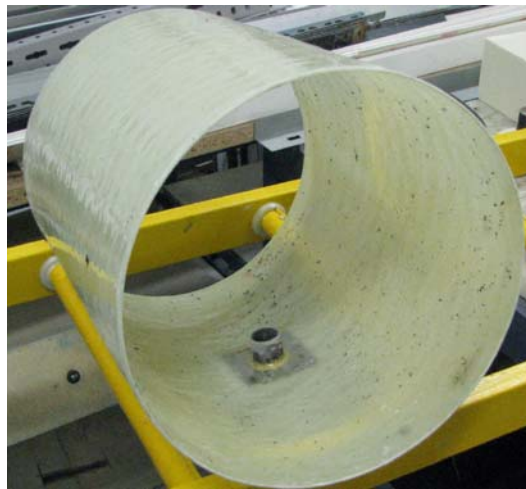
Figure 7-31 Finished hollow cylinder [2, 15, 16].
