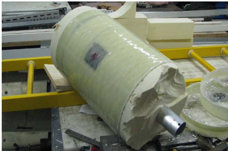
Figure 7-30 Removal of thick edges of the cylinder (results in cylinder of 400 mm length) and start of the removal of the internal PU foam [2, 15, 16].
