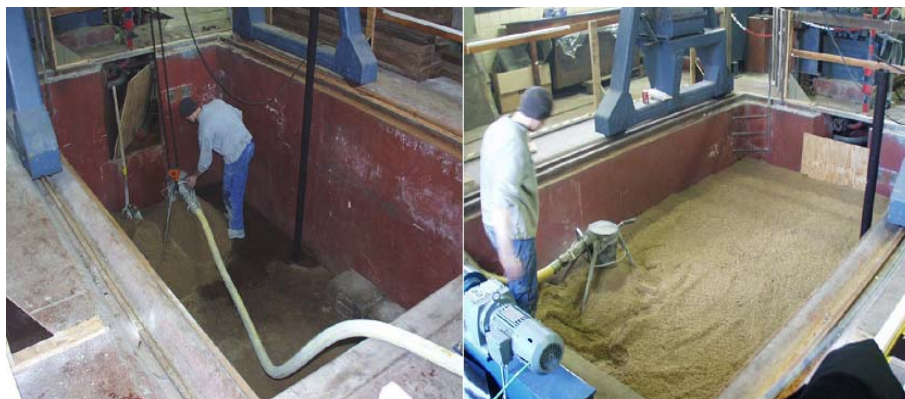
Figure 6-43 Filling the well with sand near start (left) and end (right) [14].
