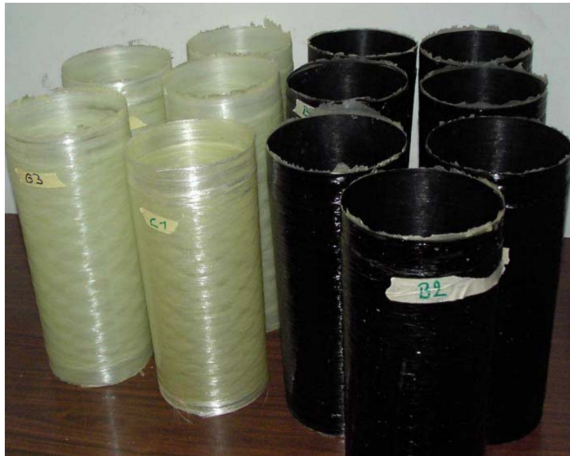
Figure 6-20 Twelve wound cylinders: five made with glass fibre and seven with basalt fibre [3].
