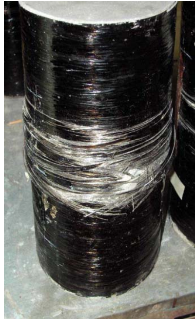
Figure 6-21 One of the tested basalt cylinders filled with concrete [3].
