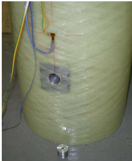
Figure 7-32 Two outer strain gauges on the hollow cylinder [2, 15, 16].
