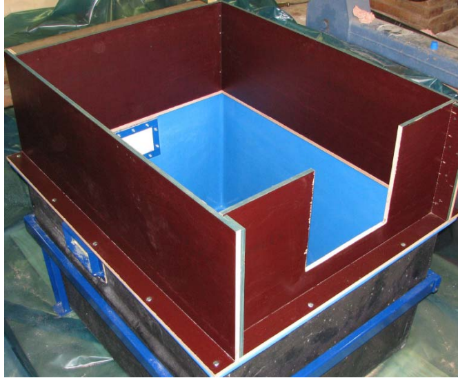
Figure 6-42 Container with added wooden frame to prevent large quantities of water splashing over the edges [14].
