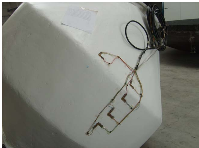
Figure 8-47 Buoy with the five pairs of outer strain gauges.
