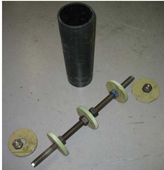
Figure 6-15 Parts of the mandrel used for the winding of cylinders [3].
