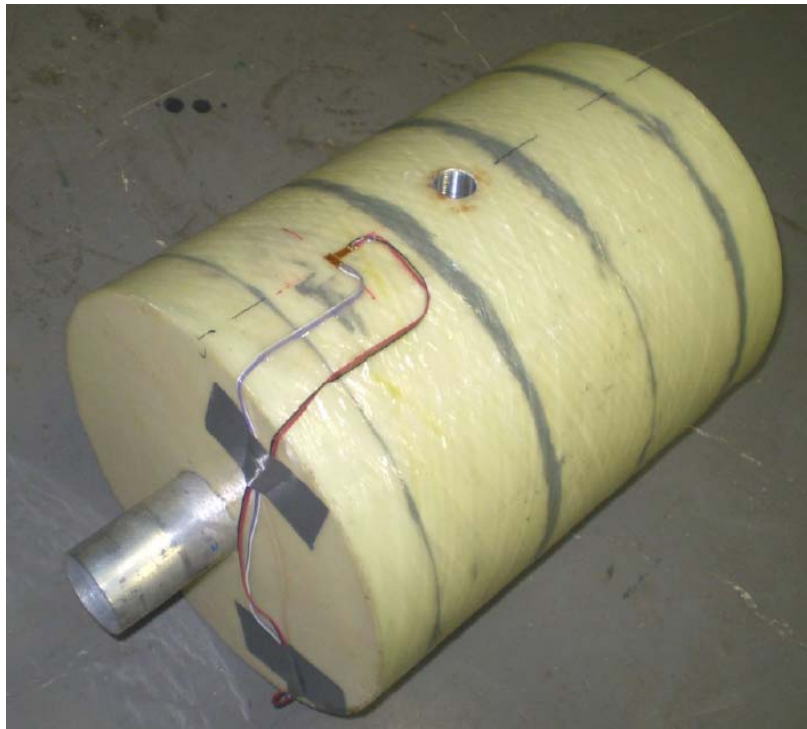
Figure 7-18 Full cylinder with two strain gauges and its preparation for one pressure sensor [2, 15, 16].
