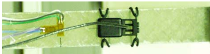
Figure 4-18 Strain gauges (left) and extensometer (right).
