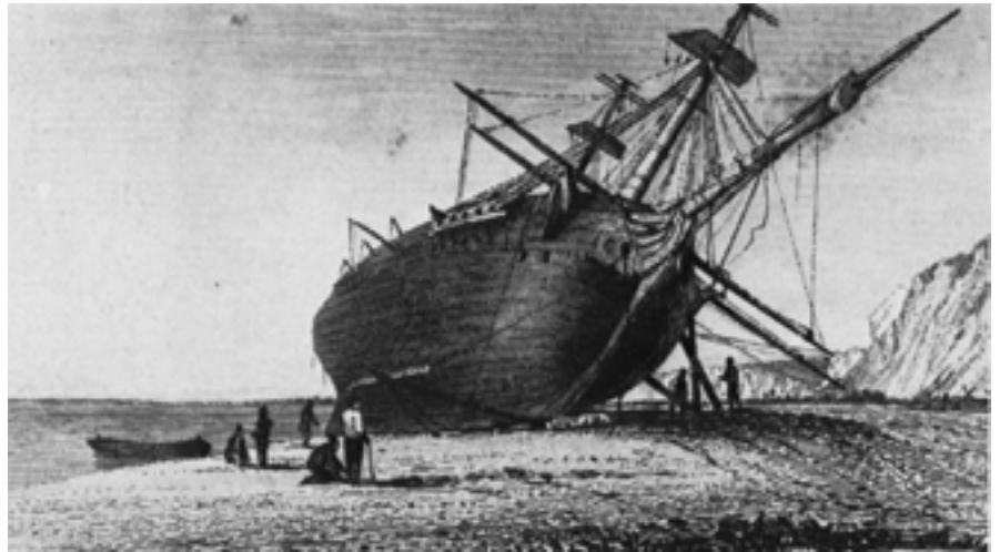
Figure 4. Conrad Martens, an official artist on the second voyage, did this drawing of the Beagle laid ashore at the mouth of the river Santa Cruz in Southern Argentina. When repairs to the hull were necessary after the ship had struck a rock, the ship was beached and the work was performed between high tides. (Image courtesy of the Beinecke Rare Book and Manuscript Library, Yale University.)
