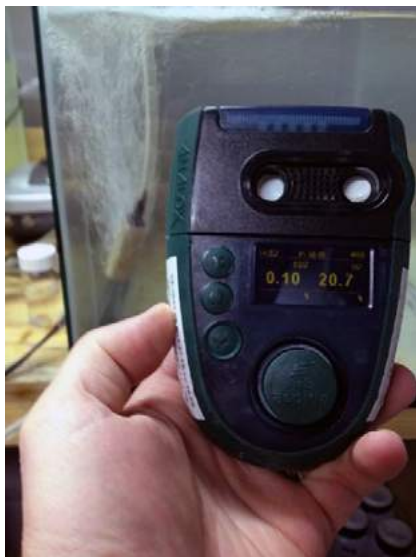
Figure 1: A handheld CO 2 sensor, typically used to ensure safe levels during submersible dives, is used to measure rising CO 2 in the cold room on the R/V Atlantis.
