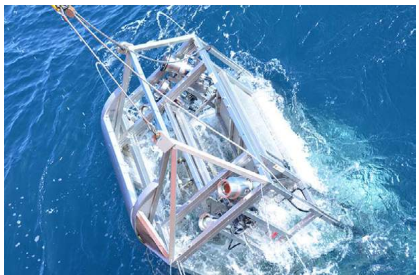
Figure 2. The Camera Epibenthic Sledge (C-EBS) is equipped with video and photo cameras. Its small-meshed nets are designed to catch primarily benthic macrofauna. Picture: Angelika Brandt.
