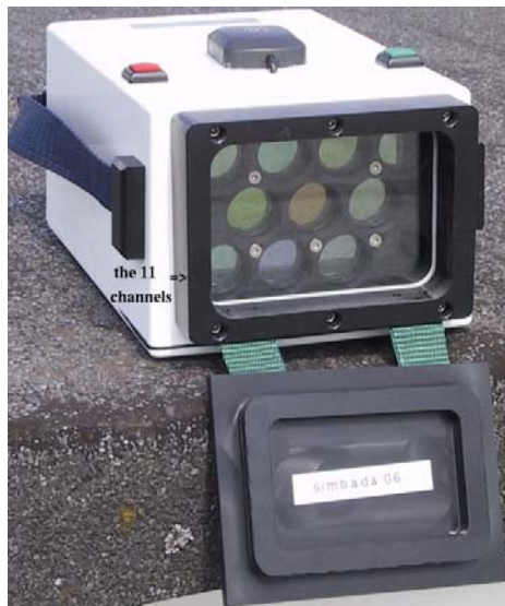
Figure 11. View of SIMBADA showing foreoptics.
