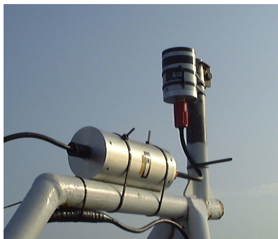
Figure 6: Atlantic sensor head for E_s(\lambda) measurements.
