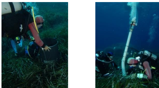
Fig 2. Set up of the cylinder enclosing Posidonia oceanica leaves (left), and airlift sampling (right). (Photos: Trainito E.)
