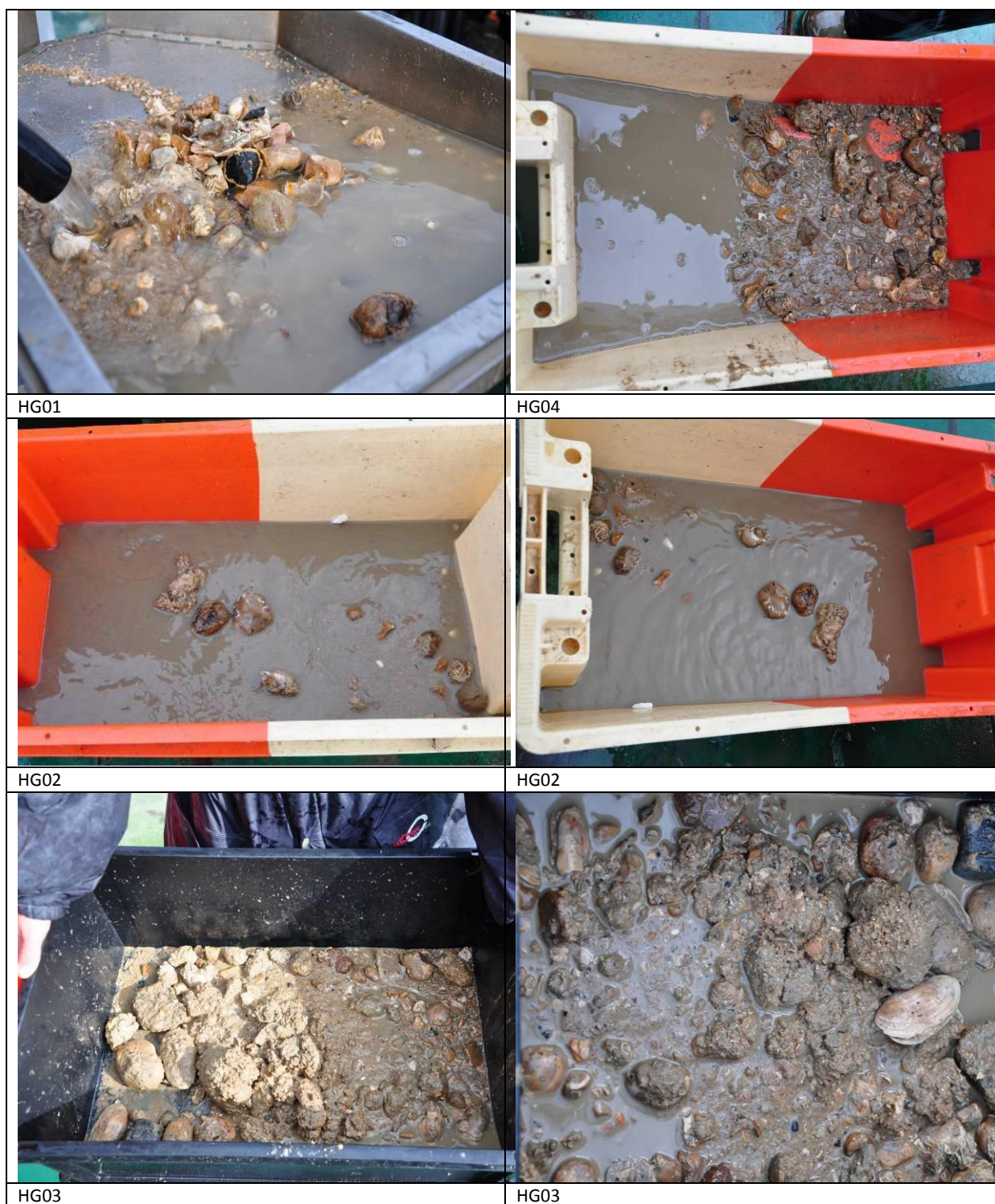
Figure 42. Mud enrichment in the gravel rich area of the barchan dunes, west of the Oosthinder sandbank, Habitat Directive area. Hamon grabs were taken during RV Belgica ST1407, for positions, see Figure 16.
