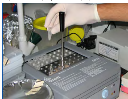
Figure 6. Samples in a thermal block at 55 °C.
