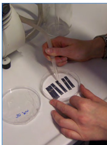
Figure 8: Drying of chips using a vacuum pump and a wash bottle.
