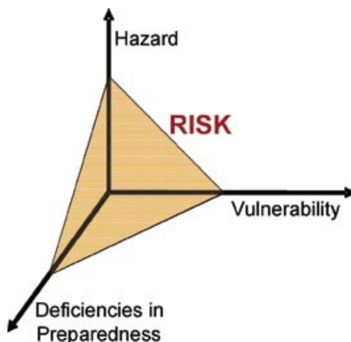
Fig. B11. The elements of risk: hazard, vulnerability and deficiencies in preparedness. The risk can be mitigated by reducing the vulnerability to the hazard and improving preparedness.
