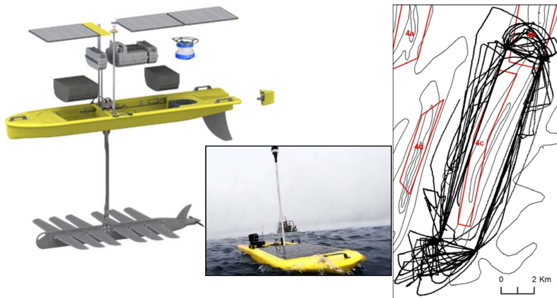
Figure 3. Left: Wave Glider SV2, Liquid Robotics. Float (payload, incl. ADCP) and sub. Right: trajectory during the period 15/4 – 6/5 2013 (see also Annex F).
