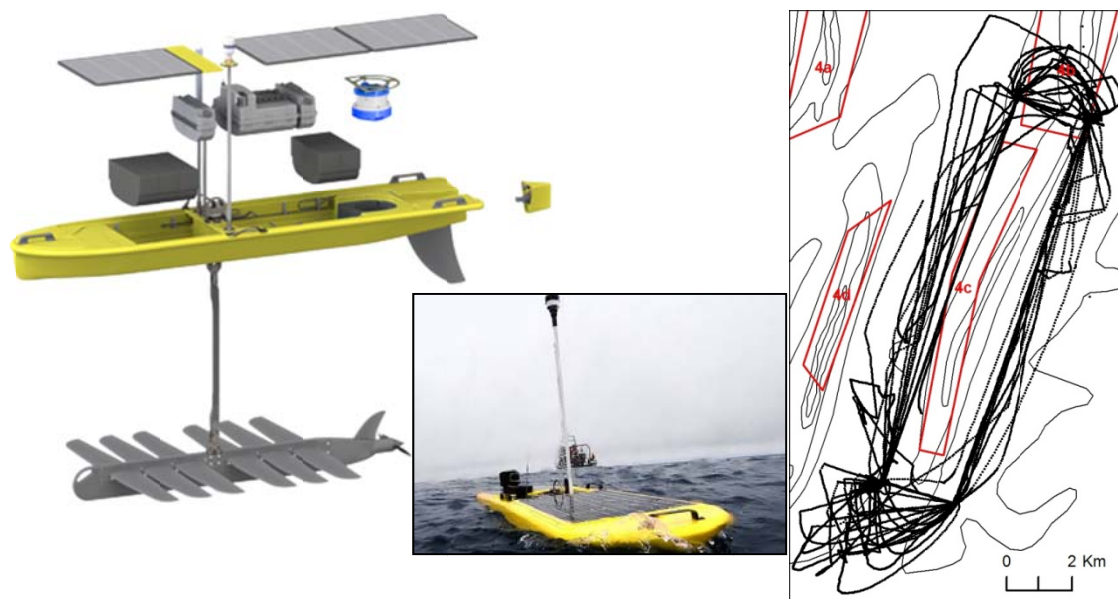
Figure F-02. Left: Wave Glider SV2, Liquid Robotics. Float (payload, incl. ADCP) and sub. Right: trajectory during the period 15/4 – 6/5 2013.
