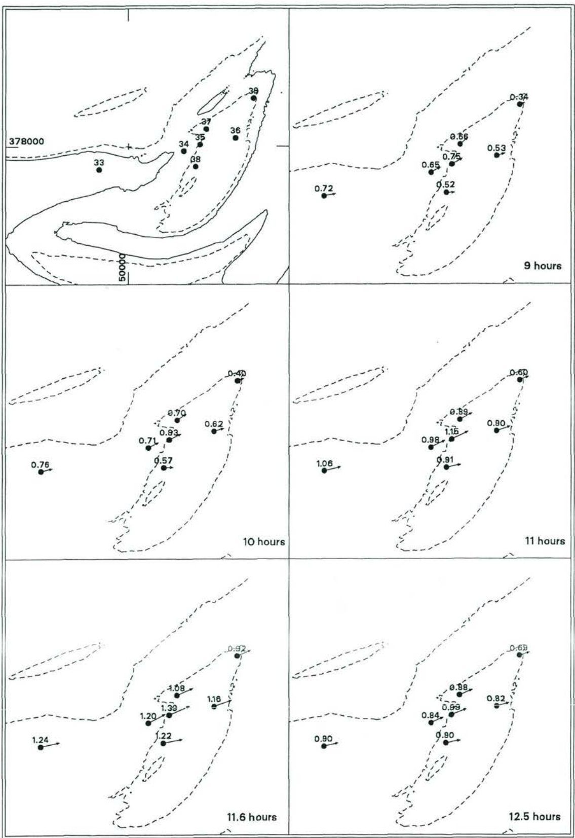
Fig. 4.54 Depth-averaged current current patterns in the flood bar channel during flood and mean tidal conditions in February 1996.
