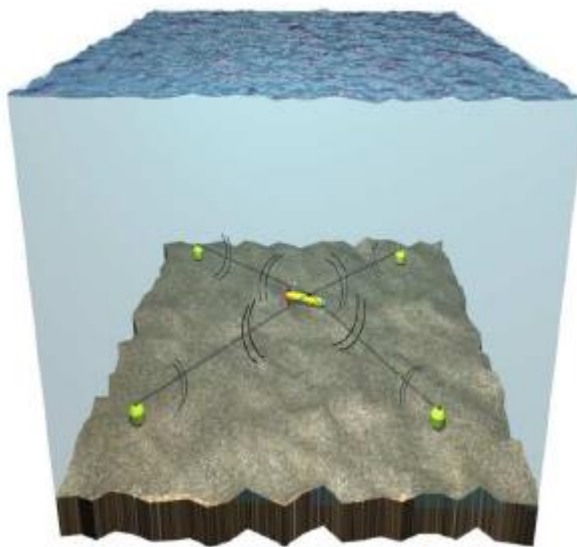
Figure 1. Principle of long-baseline (LBL) underwater positioning systems
