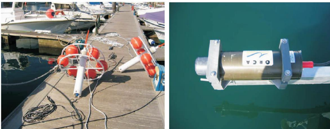
Figure 6. Left: GIB buoys before deployment. Right: GIB pinger.
