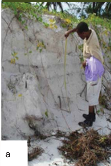
Fig. 27. Beach plain sand deposits: backshore erosion scars in siliciclastic sand: (a) at Nyali on the Bamburi shore, and (b) at the mouth of the Mdumbwe River, Kunduchi site. Photos: Y.W. Shaghude.
