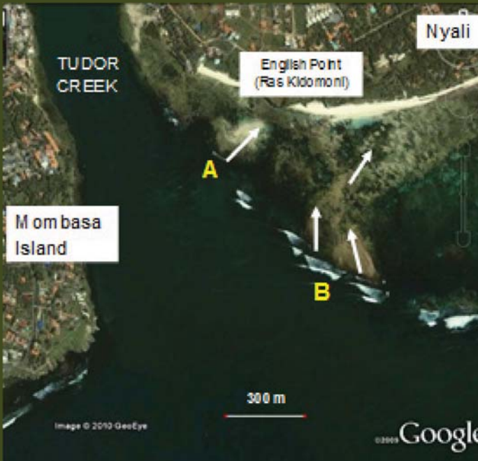
Fig. 26. Sand supply pathways from Tudor Creek to the south-western end of the Bamburi site intertidal platform at English Point; mainly siliciclastic sand transfer at A, mainly biogenic carbonate sand at B. Arrows show cross-platform sand transport directions as inferred from bedforms. Image at low water, 30 July 2007 © 2010 GeoEye. Based on Shaghude et al., 2013.
