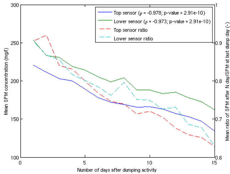
Figure 12: SSC evolution at Oosterweel in the first two weeks after sediment disposal nearby
