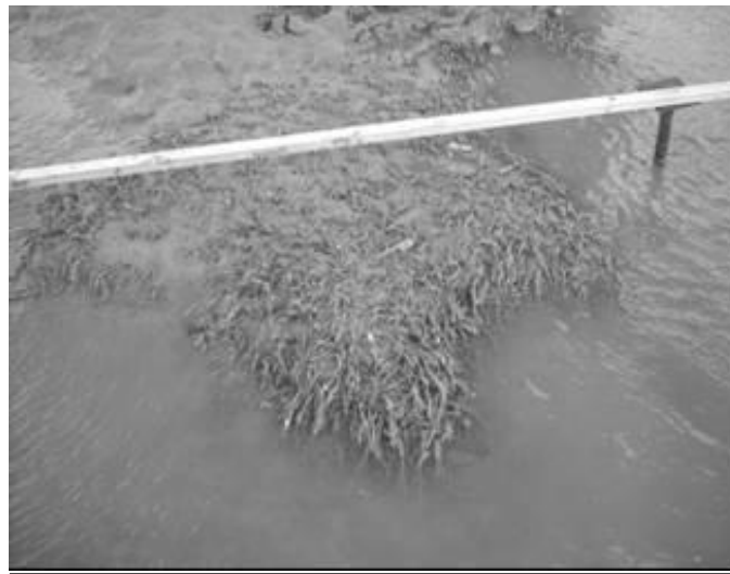
Figure 3. Methodology to determine the relative height differences of individual aggregations: the vertical distance to the horizontal conduit was measured every 10 cm.
