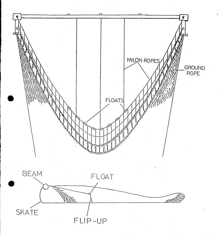
Figure 2. Upper panel: Top view of the flip-up rope (meshes of about 40 cm) and attachment to groundrope and beam.
