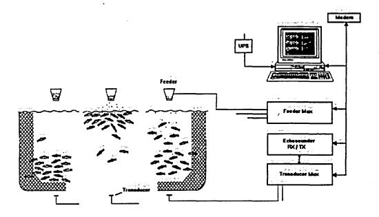
Figure 1. General configuration of the Cage-eye system. The three boxes to the right are from the top; Feeder multiplexer, Echo sounder with receiver/transmitter (RX/TX) and Transducer multiplexer at the bottom.
