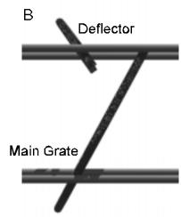
Figure 1. Oblique view (A) and side view (B) of the halibut excluder grate installed in the intermediate section of a trawl. Mesh sides of the intermediate have not been drawn but riblines are illustrated.
