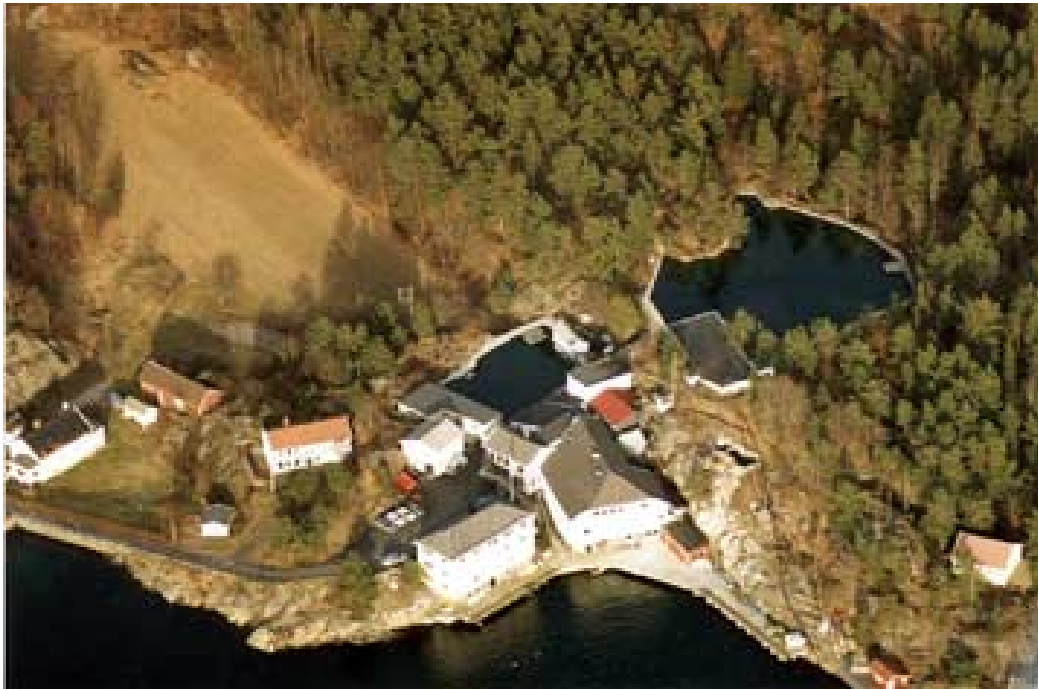
Figure 2. The two mesocosms at the Institute of Marine Research, Flødevigen Research Station, Arendal (left basin: 2500 m 3 right basin: 4400 m 3 ).
