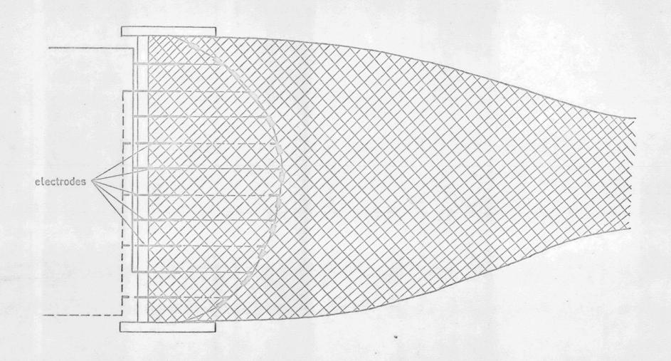
Figure 2 \_ Beamnet with electrodes
