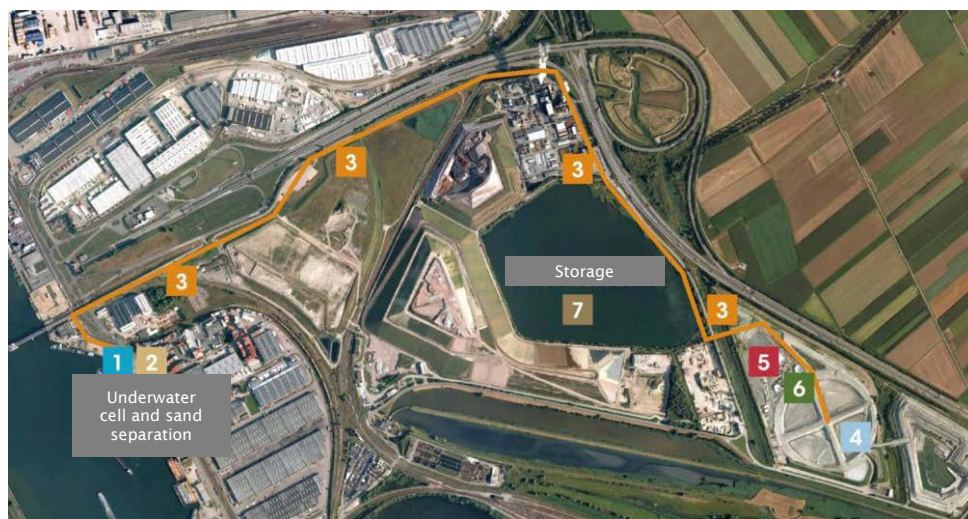
Fig. 1. AMORAS production sites: 1. underwater cell, 2. Sand separation, 3. Piping, 4. Consolidation ponds, 5. Dewatering installation, 6. Water treatment, 7. Storage.
