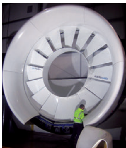
Fig. 3.19 Tidal turbine being prepared on land. The concept is being tested for use in the deep ocean.
