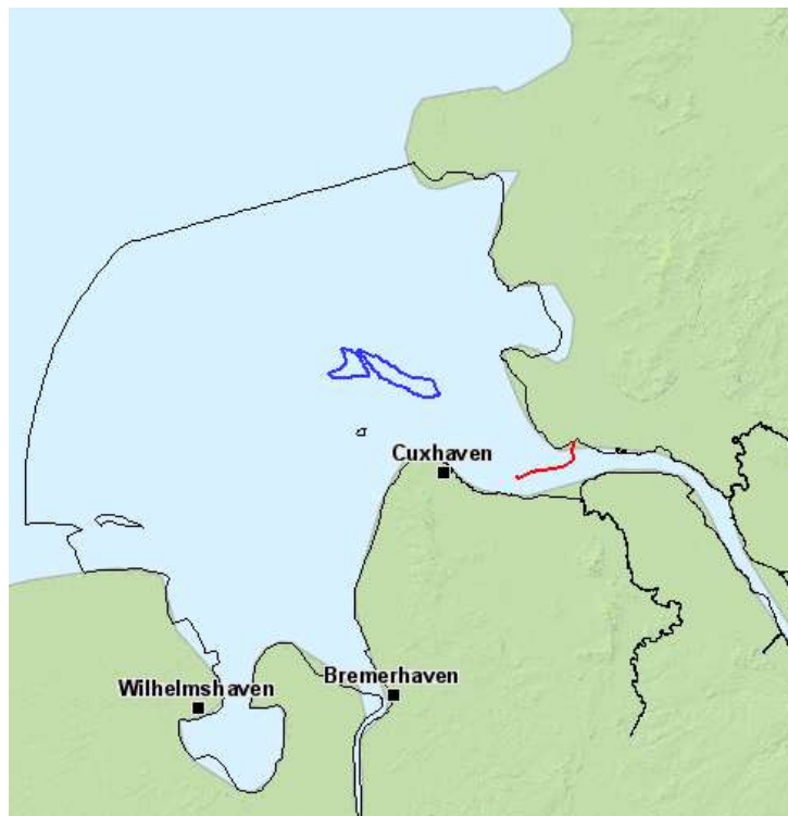
Figure 1 Overview of the Elbe estuary showing the modelled area (black line) with sketches of the expansive (blue) and linear (red) structures.
