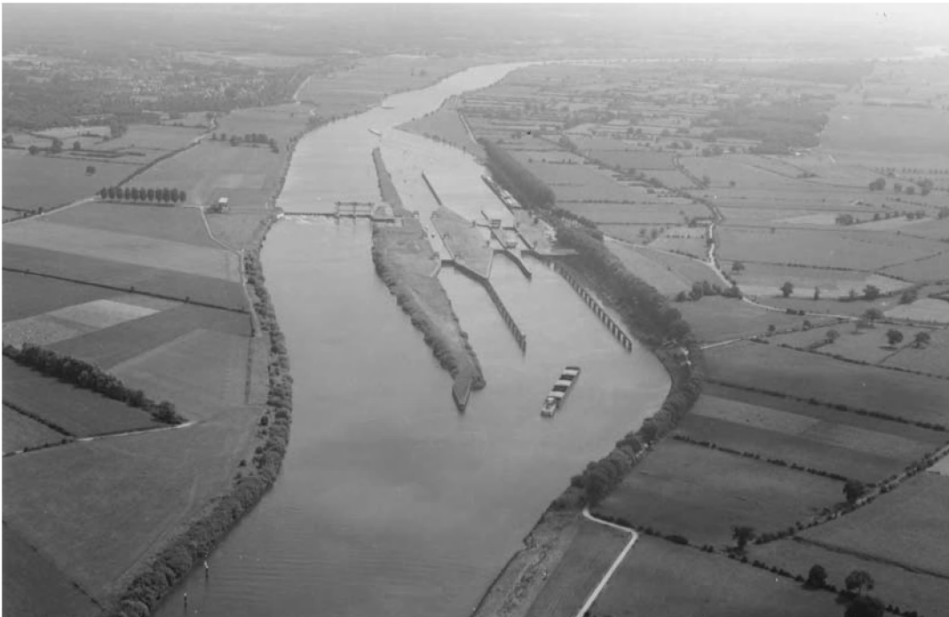
Photo 5.7 Lay out of lock complex at Sambeek on the Maas with weir (left) and 3 navigation locks
