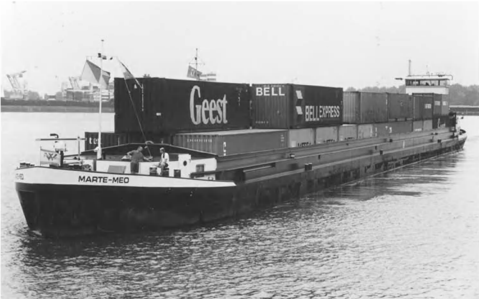
Photo 4.11 Container vessel CEMT class IIIa
