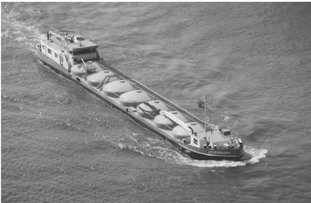
Photo 4.9 Cement tanker CEMT class IIa
