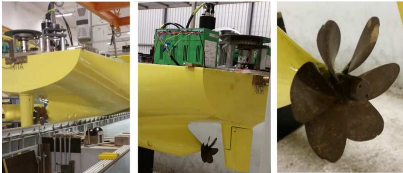
Figure 4.6 Single propeller and single rudder installed on the ship model.
