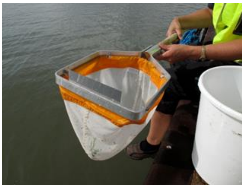
Figure 2. Scraping tool used in sampling of fouling community
