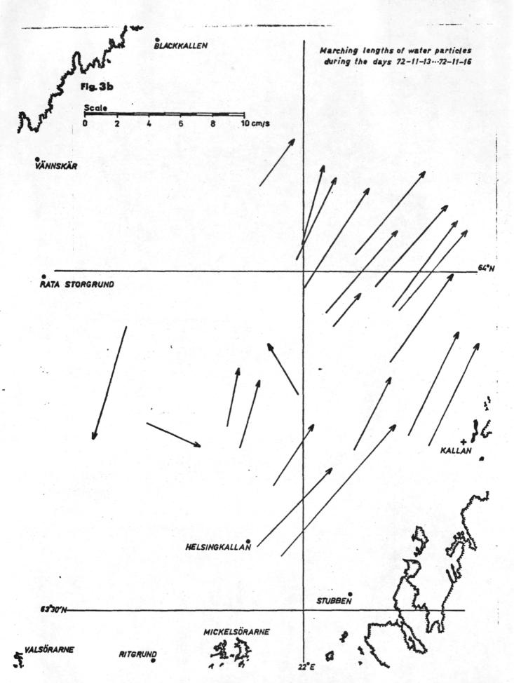
Points, where the same water masses were believed to reside, were connected with arrows. They represent the marching lengths of water particles during the interval from Nov. 13 to Nov. 16, 1972.
