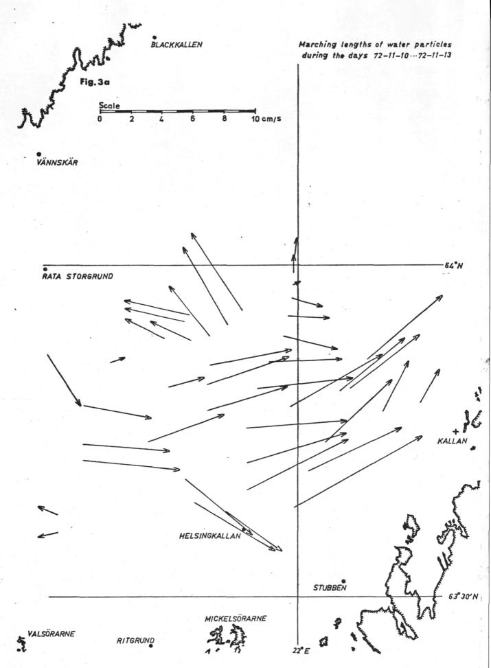
Points, where the same water masses were believed to reside, were connected with arrows. They represent the marching lengths of water particles during the interval from Nov. 10 to Nov. 13, 1972.
