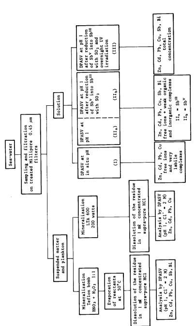
Analytical protocol to analyse Zn, Cd, Pb, Cu, Sb and Bi in suspended matter, plankton and to study speciation of metals in solution in the water column. LTA = low temperature ashing (activated  $O_2$ ).
