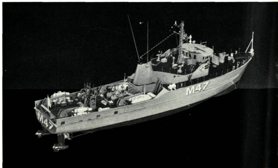
Model of 47 m Minehunter showing the Pleuger rudders for accurate manoeuvring at low speed (0-6 knots) and the layout of the sweep deck.
