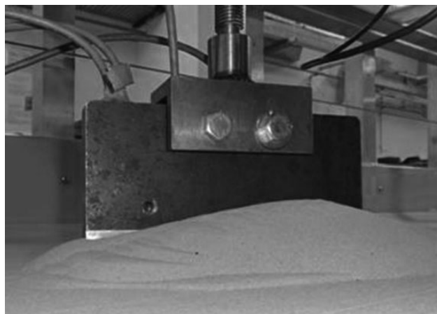
Figure 2. A demonstration of sediment failure in front of a towed penetrating object in a sand channel where there are alternating regions of resistance separated by failure surfaces.
