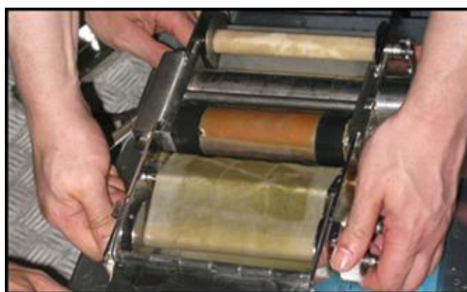
Figure 5.5. Continuous Plankton Recorder on a Dutch ferry (photo Robbert Jak/ IMARES).
