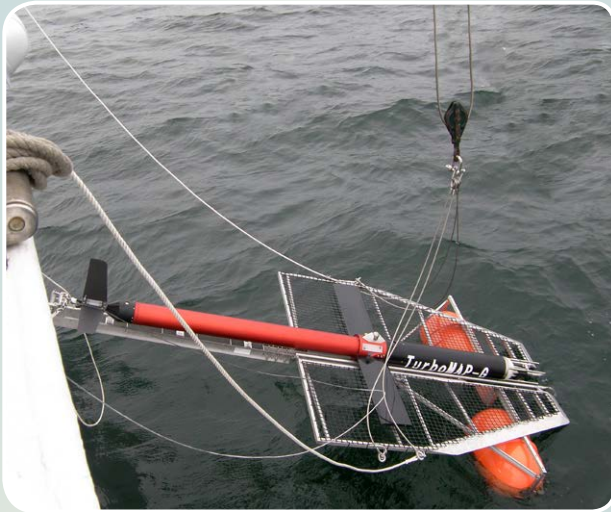
The TurboMap-G (H Yamazaki, Japan) device allows us to understand the small-scale physical hydrodynamics that control the aggregation of toxic microalgae in thin layers in the water column. Photo: H. Yamazaki.
