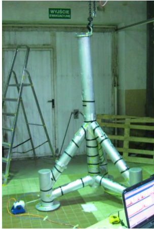
Figure 2 Tripod model in experimental setup for structural dynamics identification
