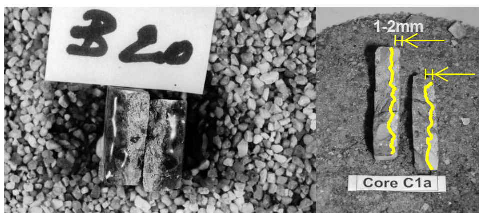
Figure 3: Example of hydrophobic action. Visual inspection by wetting a fresh cracked surface (slice thickness equals 7 mm) – core B2 (left: 1998) and core C1 (right: 2005)
