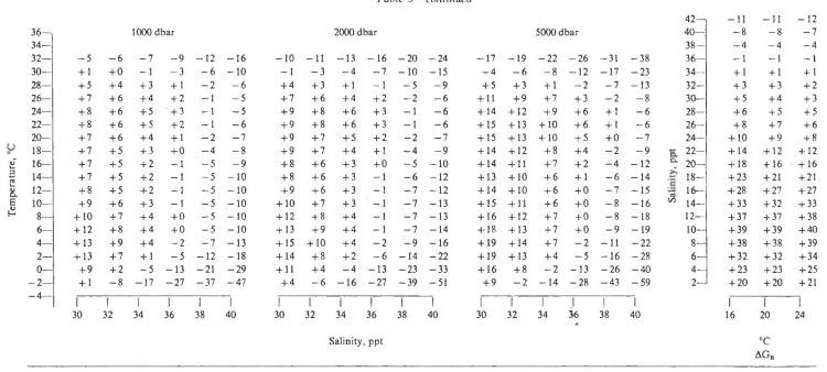
$\Delta G_B$  at the lower right of Tables 3 to 7 gives the calculated change in bottle sample salinities used for calibration purposes. See text for discussion and method of use. Dashed line encloses the region of validity of the equations as given in Table 1.
