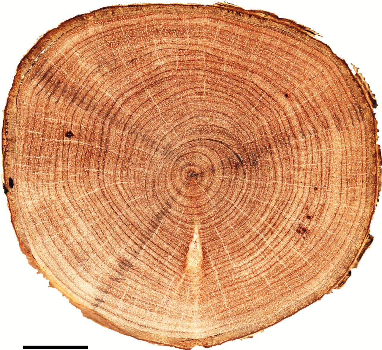
Fig 3. Transversal view of a sanded stem disc showing tree-ring boundaries with pencil marks. Scale bar = 10 mm.
