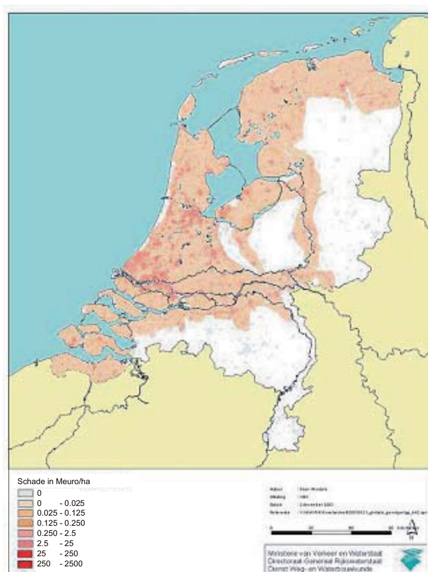
Figure 3-9 Map of damage in the Netherlands at the water depths given in Figure 3-6.
