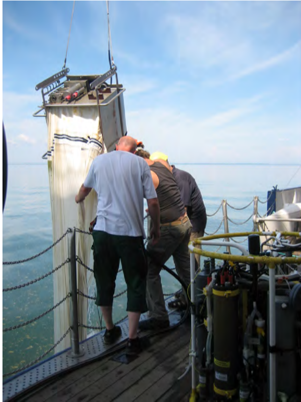
Deploying a plankton net at sea
