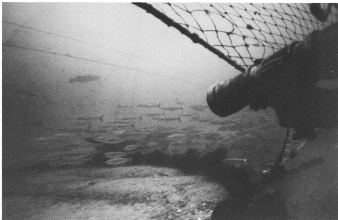
Figure 1. Photograph taken from the diver's towed vehicle showing saithe, Pollachius virens , swimming ahead of the mouth of a trawl. The low-light TV camera seen on the right is used by a diver to record the behaviour of the fish with much greater clarity than can be captured on film.
