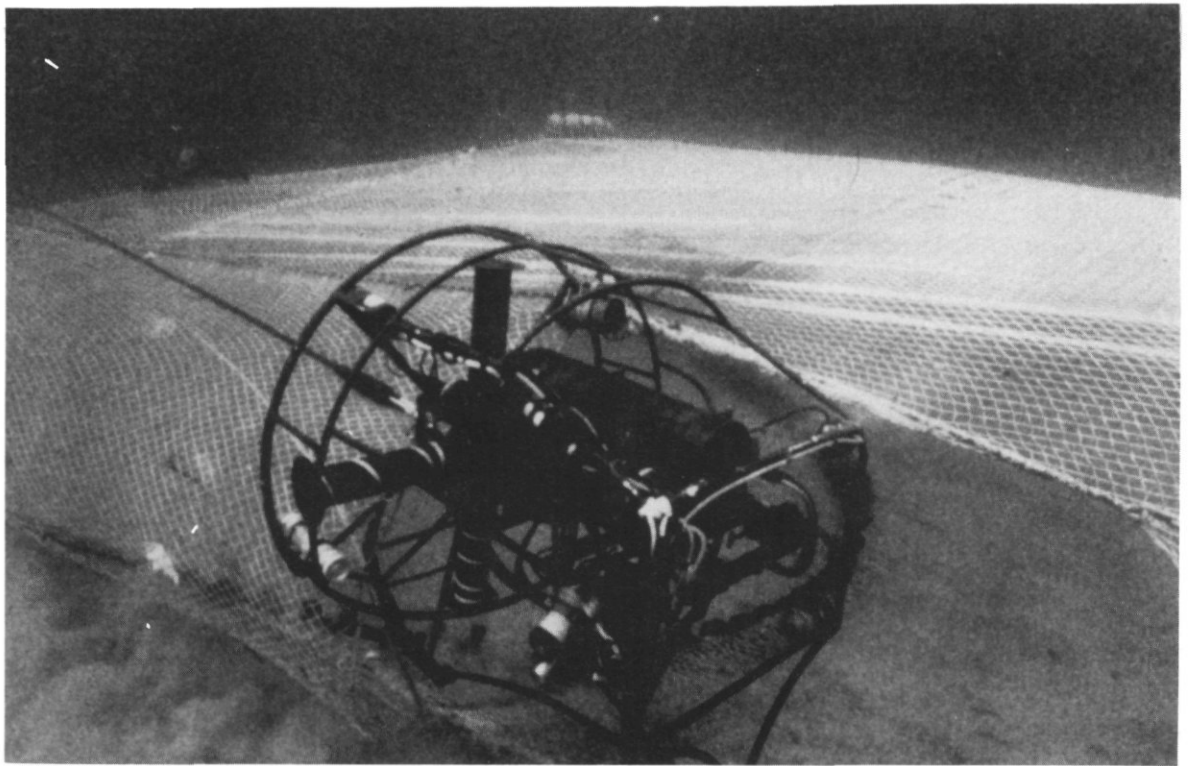
Figure 2. The Aberdeen Marine Laboratory's unmanned, towed, remote controlled vehicle alongside a net. Vertical and lateral control is achieved with Magnus rotors (spinning cylinders). The vehicle carries TV cameras, still cameras and other instruments to study gear performance and fish behaviour.
