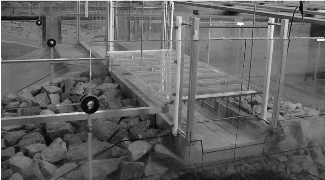
Photo 1 : Physical model set up of the walkway on top of the breakwater
