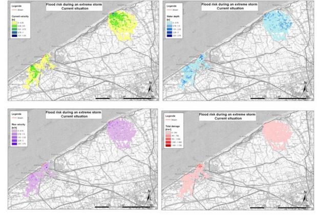
Fig. 3, 4, 5, 6. Flood risk calculations for an extreme storm under present climate conditions: current velocity [m/s], water depth [m], rise velocity [m] and total damage [€/m²].
