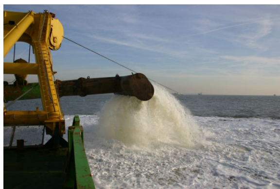
Figure 2. Detail of diffuser head (ponton Bayard II)
