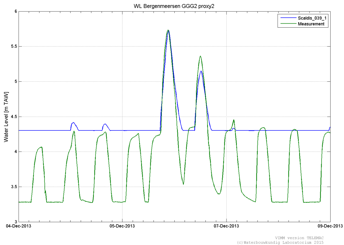
Figure 472 - Calculated and measured water levels at Bergenmeersen CRT2 (Scheldt)
