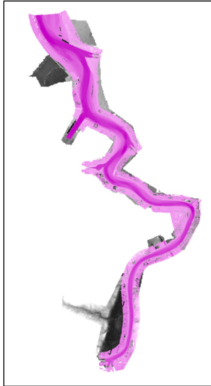
Figure 12 - Bathymetry lower Sea Scheldt. Beneden Zeeschelde. The purple coloured zone is part of a topo-bathymetric dataset from 2011. The grey area is the back is part of the DHM Vlaanderen dataset from 2007.
