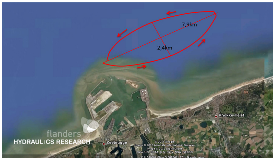
Figure 6 - Tidal excursion length based on the M2 component near the port of Zeebrugge
