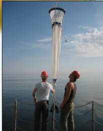
WP2 plankton net deployed in the Baltic Sea.
